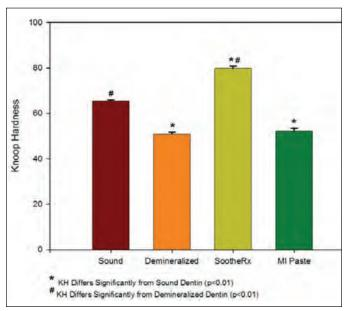
Figure 4. Surface microhardness for each treatment group.
