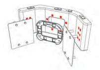
MDP with central LEDs at full power + polarizing filter, lateral LEDs at low power + diffusers. With Flexipalette contrastor and retractors.
