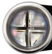
The Valo curing light head, showing the arrangement of the LEDs
